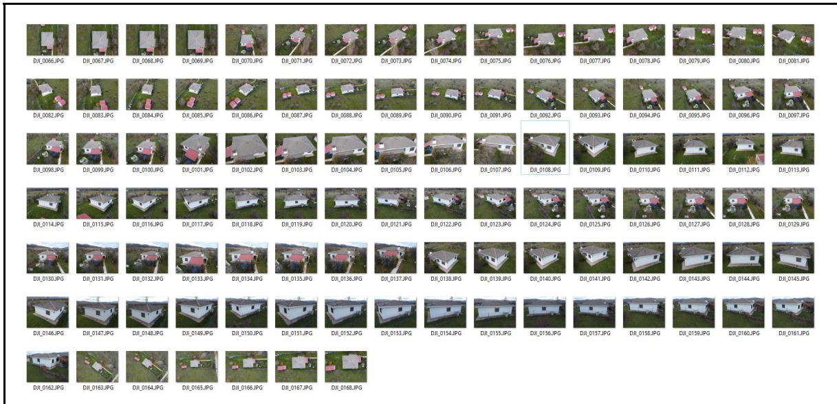
Figure 19. The full collection of the obtained photos in this preliminary test flight in study case 3 in Madrid Autonomous Region. The camera tilt angle was set remotely with 1° accuracy. Observe that the building is seen completely in every frame.
