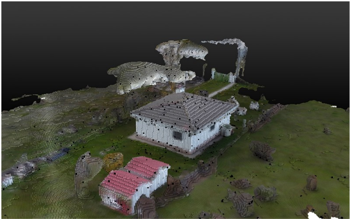
Figure 28. A voxelized version of study case 3 in Madrid Autonomous Region, with a voxel size of 10 cm, rendering a large number of objects. Colour gathered from pictures is used as reference for material assignment in further steps.
