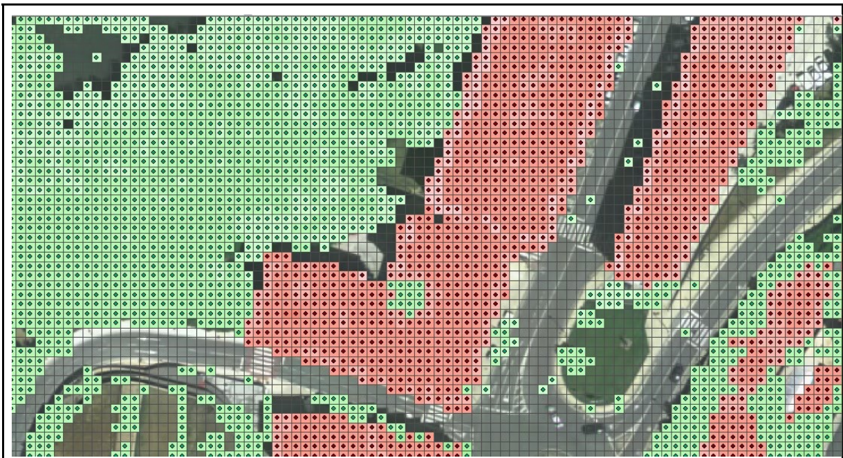
Figure 7. Segmentation of returns 1 and 2 of classes 4, 5 and 6 into 2D space using a 2x2 regular grid, showing the occupancy by vegetation (in green) and buildings (in red). This is a raster map generated in ArcGIS from the x,y,z list of voxels containing the LIDAR data.
