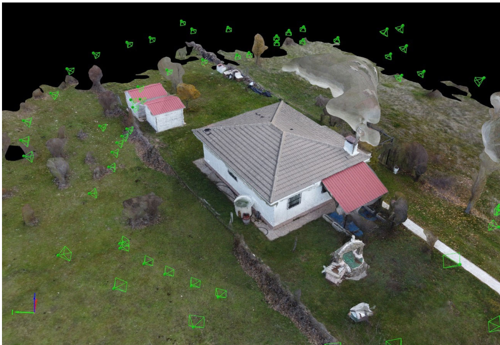
Figure 24. A high level of detail was achieved with just 95 images in the study case 3. However, some artifacts and inconsistencies are observed. These were edited in the 3D editing platform 3DSMax.
