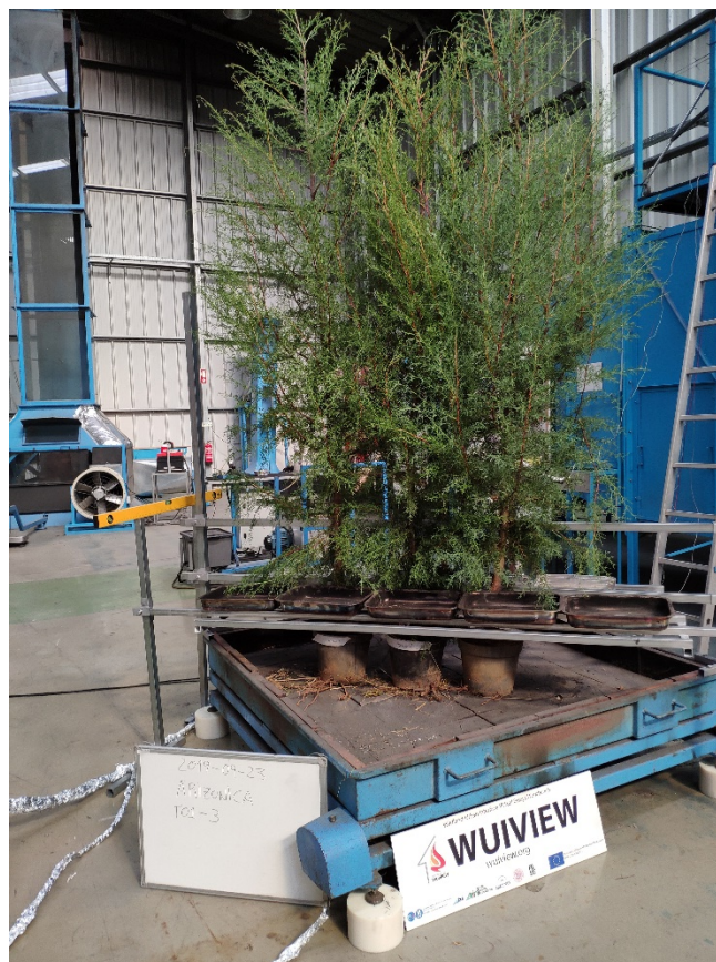
Figure 6 – View of the platform with the final setup for one of the tests, with 3 trees fixed to it.
