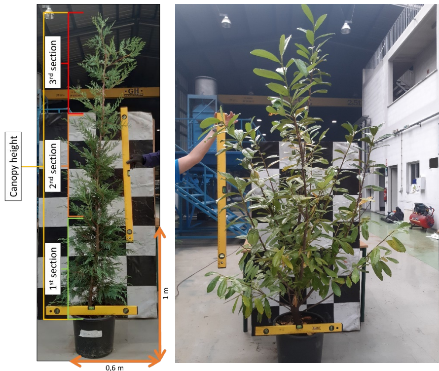
Figure 9 – Front view of a Cupressocyparis leylandii (left) and a Prunus laurocerasus (right) specimens. The horizontal rule is 0.6 m long; the vertical rule is 1 m long. The side of the chessboard reference square is 0.25 m long.
