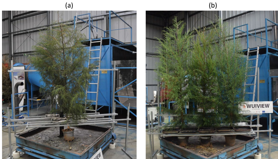
Figure 11 – Tests configuration: (a) 1-tree configuration, (b) 3-trees configuration
