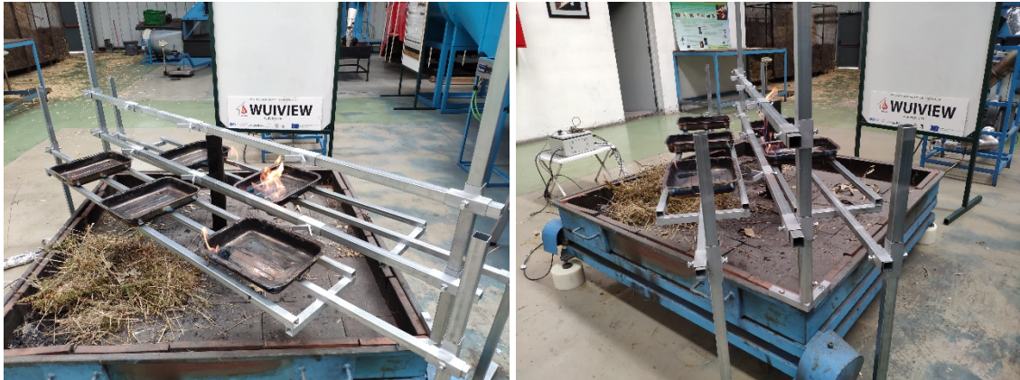
Figure 5 – View of the 2 support devices built for the combustion table.
