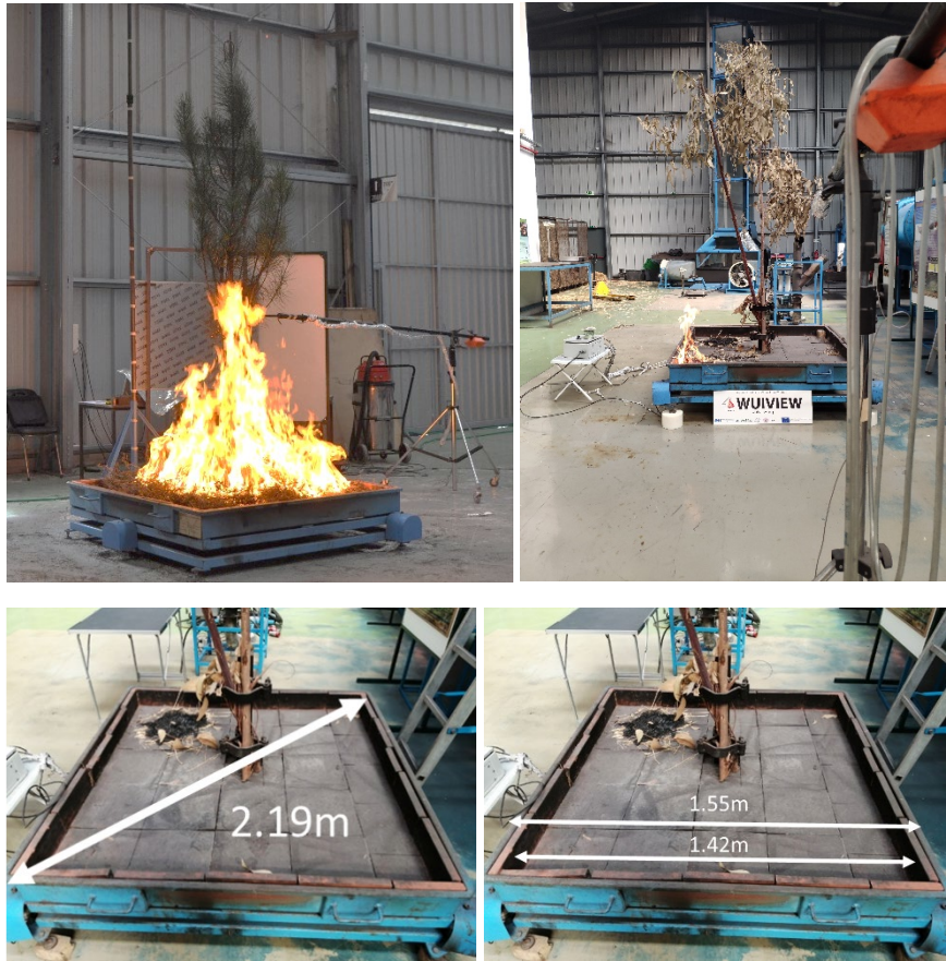
Figure 3 – ADAl's Tree Combustion Platform, with dimensions.
