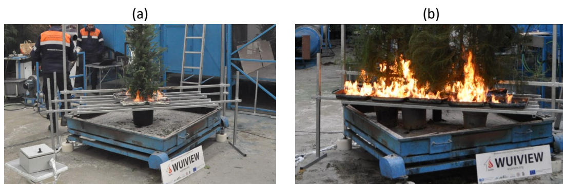
Figure 12 – Ignitions configuration: (a) 4 trays on 1-tree setup and (b) 9 trays on 3-trees setup.
