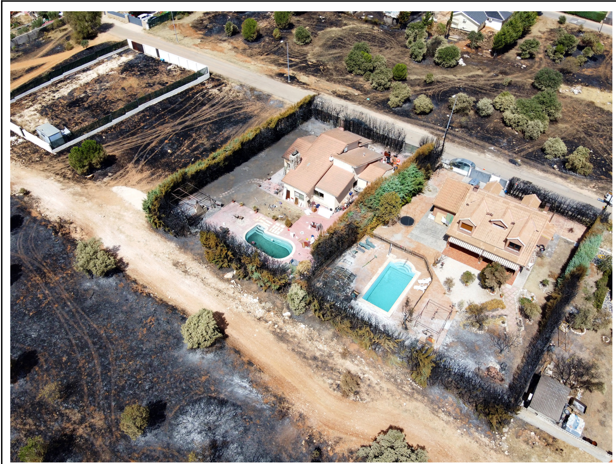
This drone picture shows a general view of the impact of fire front in the first rank of houses and green hedges. It is observed the role of these hedges in propagating the fire inside the settlement and how they contributed to the ignition and combustion of other objects and materials, such as pergolas and green houses (in the left-South corner of each parcel) and the affectation of houses. The angle formed by the main axis of propagation is clearly visible (wind blowing from WSW). In case of a wind blowing straight from the South, most likely the fire penetration could have been much more effective, through green hedges and gardens, complicating noticeably the whole event. The East limit of the community presents higher fuel loads and in case of a South wind, it is expected that the fire front could have increased the intensity even more.
