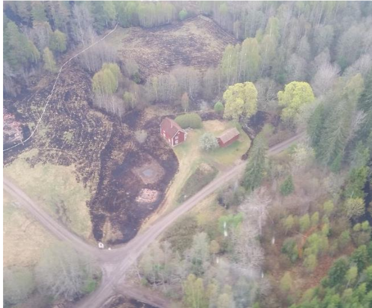
Figure 13. An example in which a low-intensity fire in a maintained lawn has carried the fire to the dwelling without subsequent ignition. The maintained lawn has prevented the fire to be carried to the outbuilding. Photo: Anders Granström.
