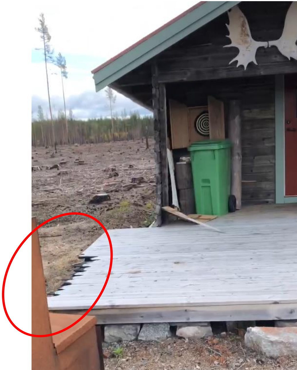
Figure 10. Example of low-intensity fire ignition by flame impingement of a wooden deck, in this case followed by extinction.
