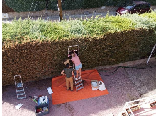
Figure 4. Process of collecting the fuel in the upper incision. Notice that the most external foliage was withered as a consequence of the exposure to radiation. The left site was the closest to the fire.
